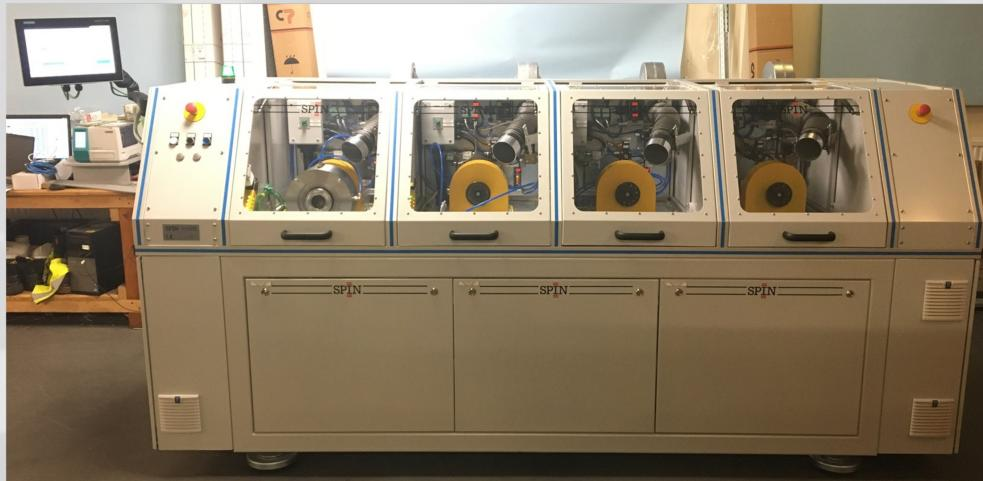
The test rig is comprised of four individually controlled test chambers. Each test chamber has its own safety interlocked access with a dedicated test programme that can run
